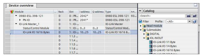
Now set the I/O addresses which you want to use in your PLC program (please refer to <u>chapter 6</u> for the data format). With a right click on the module/properties you can open the port configuration. Here you can change the general IO-Link settings for this port.
