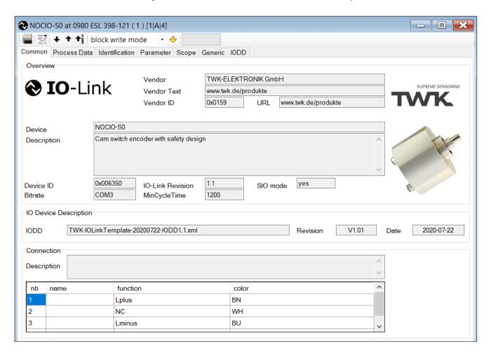
After changing one of the parameter you have to download the new configuration via the download button on the top. Please don't forget to set the parameter storage behaviour in your port configuration (see <u>chapter 7.2</u>)
