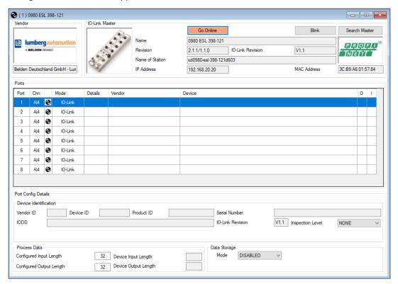
Now every device which is in the hardware catalogue can be inserted via drag and drop into the ports
