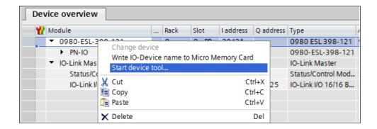
In the device tool you have to import the master description (available via the button "TMG web") and the IODD of the NOCIO. Afterwards both device are listed in the hardware catalogue.
