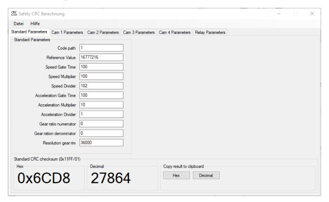
The register "Standard Parameters" is used to calculate the checksum 11FF over the encoder parameter. Registers "CAM 1-4 Parameters" is used to calculate the checksum 30FF/01-04 over the cam parameter. Register "Relay Parameters" is used to calculate the checksum 30FF/05.
