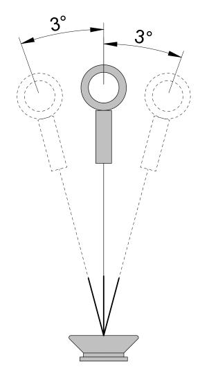
Note: The cable exit should be downwards or sideways. The cable must be extracted rectilinearly with reference to the housing (deflection max. 3° in any direction admitted).
